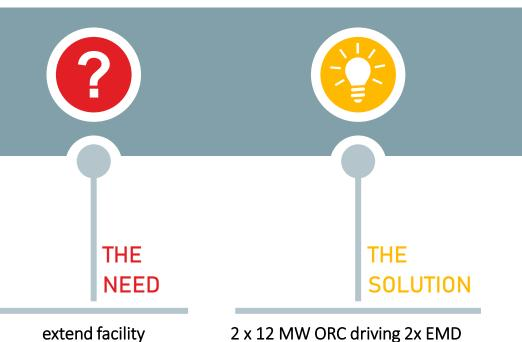
pumping capacity by 652+ MMSCFD (70% of existing compression capacity) compressors of 10 MW each (extra 4 MW to cover station auxiliaries) for 25% of the extra power required +1 new GT for the 45% of extra power.
