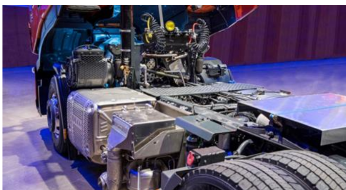
Figure 1. The prototype of a waste heat recovery system on board of a long-haul truck. Courtesy of AVL GmbH.
