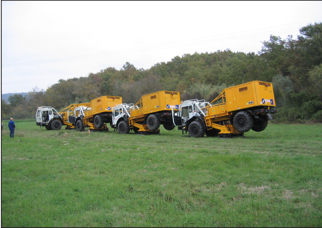
Vibroseis fleet in operation during an active seismic survey for the DESCRAMBLE project
