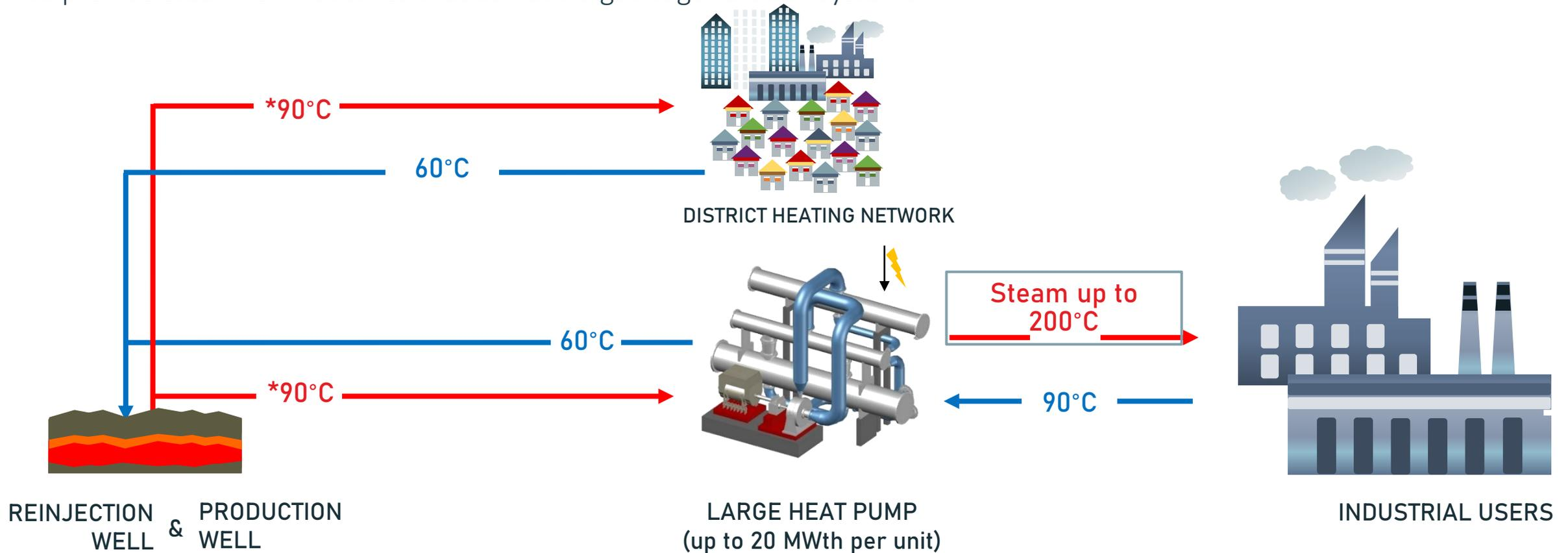
\*In case of higher temperature from production well, District Heating can be fed by Large Heat Pump discharge (cascade configuration)
