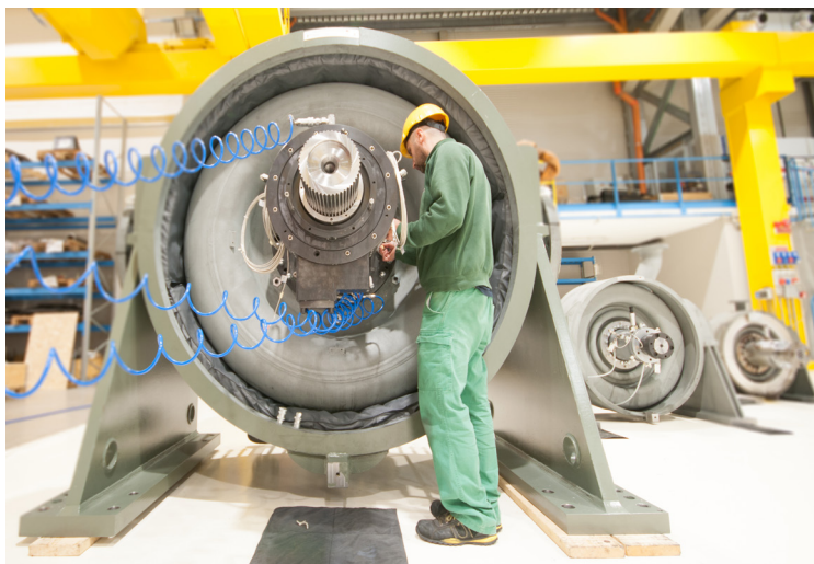
14 MW turbine assembling at Turboden workshop.
